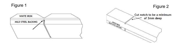
High pressure abrasive water jet cutting is preferred cutting method. Thermal cutting using an oxyacetylene torch, Arc-air or plasma is NOT recommended due to high localized heat input and high risk of cracking and delamination.
